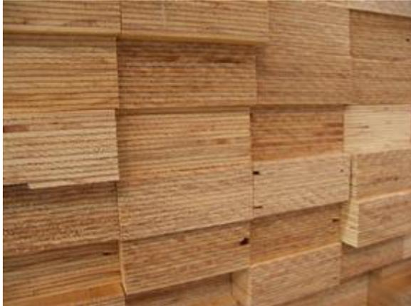
Laminated veneer lumber (LVL) is primarily used as a structural beam, rather than as a panel as in the case of plywood. Structural LVL is manufactured in a similar manner as plywood, the main difference being all (or most) of the veneers have their grain aligned longitudinally, rather than alternating perpendicular and parallel to the length. Structural LVL is manufactured with A bond gluelines and to a quality controlled manufacturing specification or 'recipe'!
