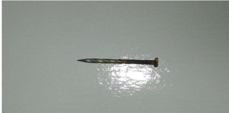
**FIGURE TWO: Corroded Poorly Galvanised Nail – Extracted from Plywood Cladding – Unsuitable for Use in Exposed Treated Plywood**
