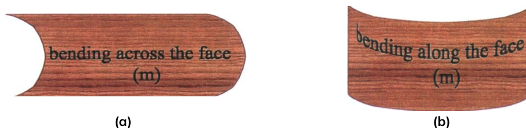
Figure 4-1: Plywood sheet bent in the easy direction (a) and hard direction (b)
