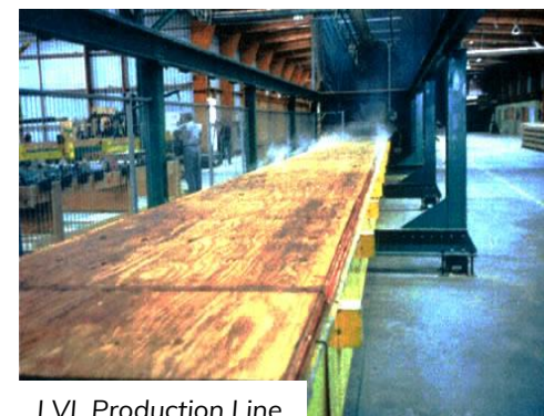
LVL Production Line
