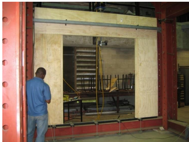
Figure 8-5: Typical Portal Frame with Discontinuous Plywood Joints
