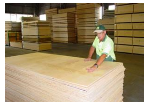
After trimming, sanding and branding, plywood panels undergo a final inspection for face quality
