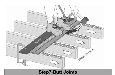
At the top centre of each KlevaKlip upright you will see a notch. This notch is designed to line up with each your butt joints. If the board is going to have a butt-join, please ensure that the end of the board finishes in the middle of this notch.
