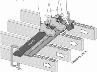
At this point, foot-pressure can be fully put across the board, pushing it fully down on the clip, and you can use the fixing tool to lock the board into the clip.
